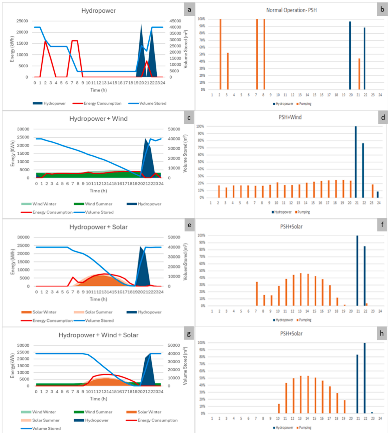
Fig. 12. Scorrídos system behavior with renewable hybridization and percentage of pumped-storage hydropower operation, for V = 40,000 \text{ m}^3 : a) Hydro operation; b) Example of daily operation for hydropower; c) Hydro+wind operation; d) Daily operation for hydro+wind; e) Hydro+PV; f) Daily operation for Hydro+PV; g) Hydro+Wind+PV; h) Daily operation for all sources.
