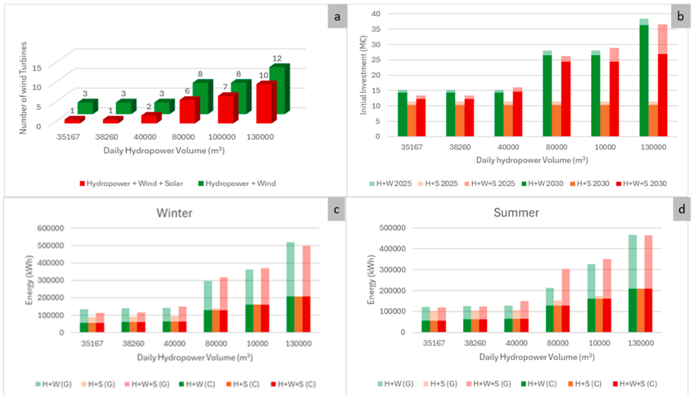
Fig. 14. Number of wind turbines installed for Scenarios 2 and 4 for different hydro volumes; (b) Initial investment in 2025 and 2030, for each solution; (c) Daily energy consumption(C) and generated (G) for each solution in winter; (d) Daily energy consumption (C) and generated (G) for each solution in summer.
