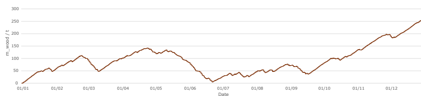
Figure 43: Cumulative available dried wood for the combined site SSR, simulated with HY4RES V2.
