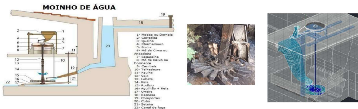
Figure 7. Schematic view of the old Moinho do Salto mill building showing the transition from the historical vertical wooden water wheel to the modern cross-flow turbine system.
