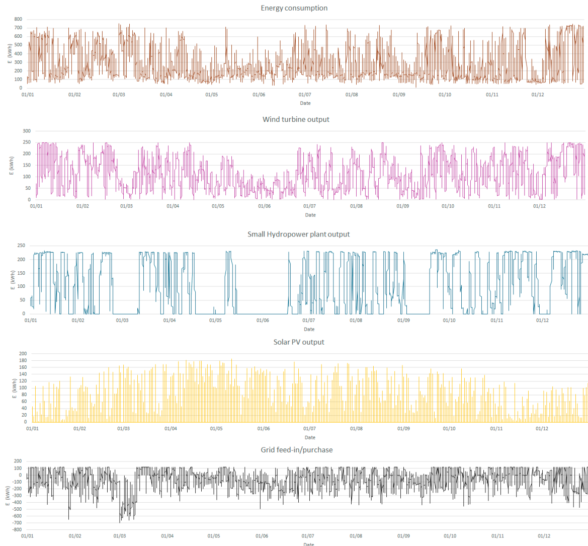
Figure 3. Hybrid energy solution with grid connection and without storage energy system—energy balance of different resources.
