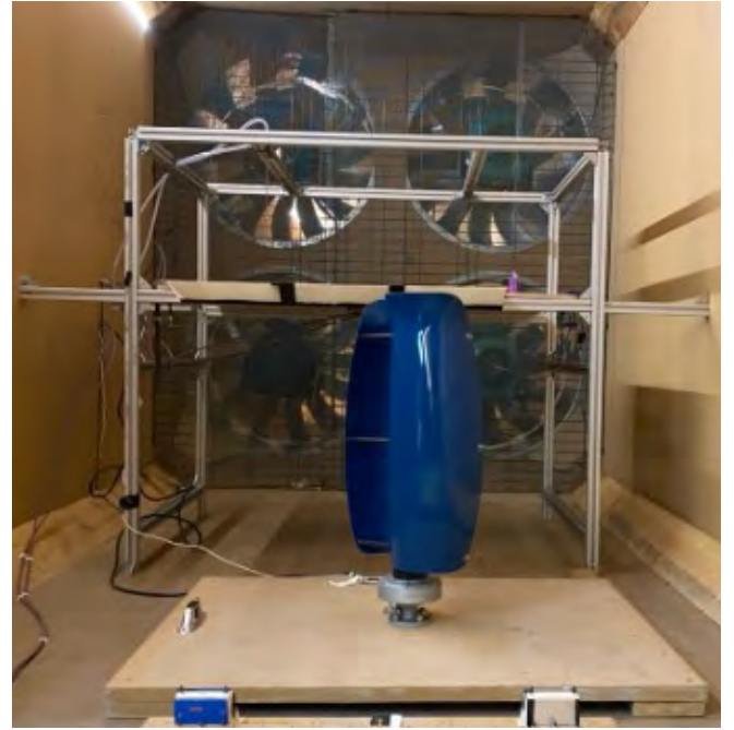
FIGURE 6: VAWT characterization inside the wind tunnel.
