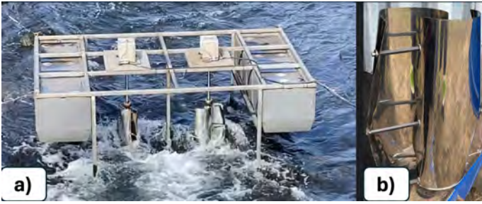
FIGURE 5: a) Hydrokinetic floating platform and b) Drag-based Savonius VAHT.
